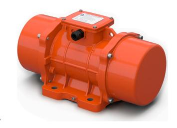
The vibrator bodies, bearing flanges and shafts are FMEA designed and manufactured from a premium aluminum alloy, cast iron and steel alloy to withstand heavy duty applications. Vacuum-impregnated windings and Class F insulation materials increase reliability and durability.
